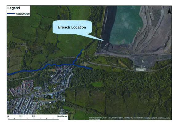
The worst case scenario is if a breach occurred at Location 1 approximately 1.75 million cubic metres of water would be released within approximately 2 hours. This would result in
